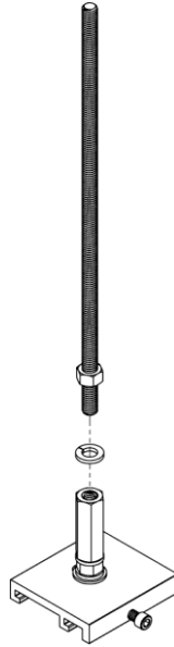
Figure 305: Level by Threading the 1/2" Coupling Nut Further On or Off of the Threaded Rod
