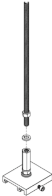
Figure 135: Thread the Ceiling Bracket Assembly onto the Threaded Rod a Minimum of Four Complete Rotations
